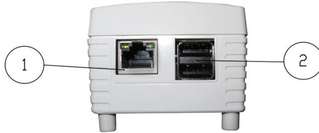
**Fig. 1: BiEasy Box connection possibilities (side view)**
