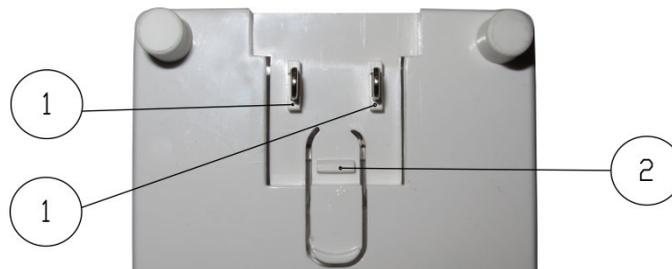
**Fig. 2: BiEasy Box connection possibilities (base view)**
