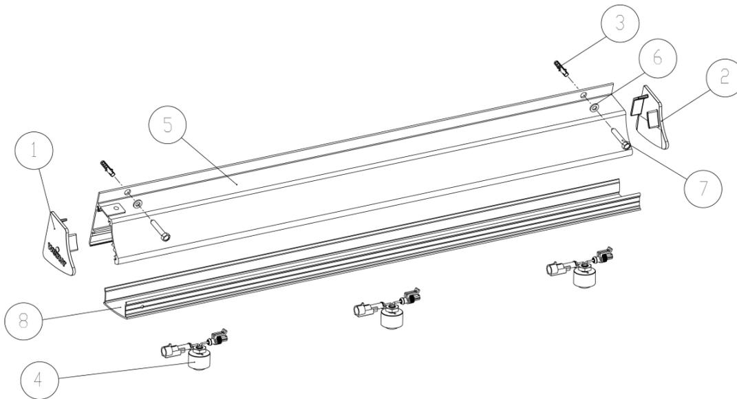
Figure 3: Exploded drawing of the LED light bar
